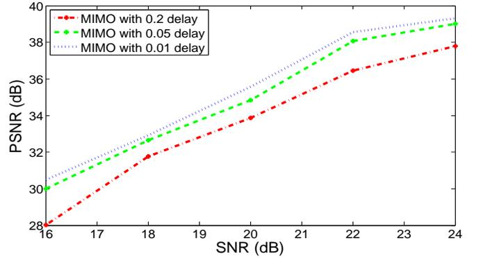
**Fig. 4.** Performance of content aware transmission scheme on Mobile CIF sequence at different feedback delay.
