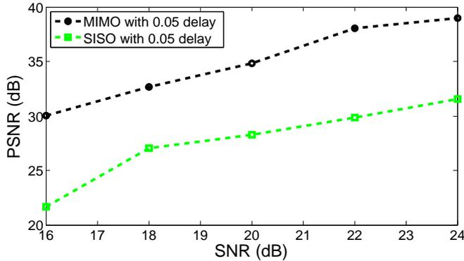
**Fig. 5.** Performance of content aware transmission scheme on MIMO and SISO at same feedback delay
