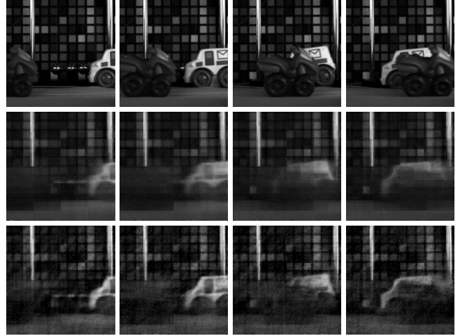
Fig. 2: Example reconstructions from the ‘‘Two Cars’’ sequence: 1 st row represents the original frames; 2 nd row represents the reconstruction through CS-MUVI [6] and 3 rd row corresponds to our proposed method.
