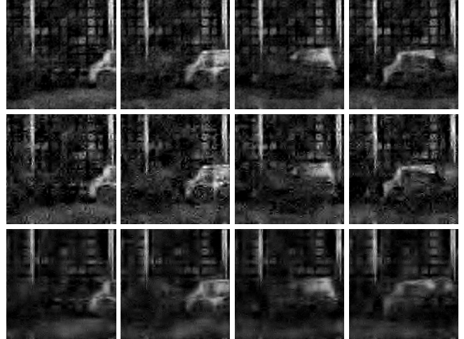
Fig. 4: Initial reconstruction of our framework (“Two Cars” sequence): 1 st row shows results (PSNR = 20.73dB) when the first row of \Phi is constructed as defined in 4.1.1; 2 nd row shows results (PSNR = 19.27dB) based on SMV instead of MMV when the first row of \Phi is constructed as defined in 4.1.1; 3 rd row shows results (PSNR = 19.10dB) when the first row of \Phi is constructed using i.i.d. Gaussian random values and the MMV approach is used.
